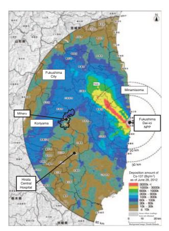
Fig. 1. Deposition amount of  $^{137}\mathrm{Cs}$  on the ground surface within a 80 km radius of the Fukushima Dai-ichi NPP (fifth airborne monitoring survey, as of June 28, 2012).<sup>2)</sup>
