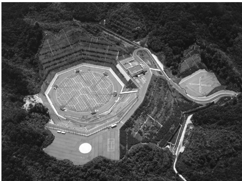
Fig. 5. Bird-eye view of the MU radar in Shigaraki Shiga in Japan. In the circular antenna area with diameter of about 100 m there are 475 of 3-element crossed-Yagi which are arrayed to make up 25 groups, each group with 19 elements (arrayed in hexagon-shape area) and each element has a transmitter-receiver module. The total system is computer-controlled so as to make it possible to steer the beam to almost any direction within 30^\circ of zenith angle in an interpulse period of one millisecond. All of the modules are shared and stored in the 6 booths around the antenna area. The area is valley-shaped surrounded by the metal-net fence as tall as 10 meter preventing radar waves from being transmitted to and returned from near-by mountain (as clutters) in low elevation angle. The shortest range resolution is about 150 m.
