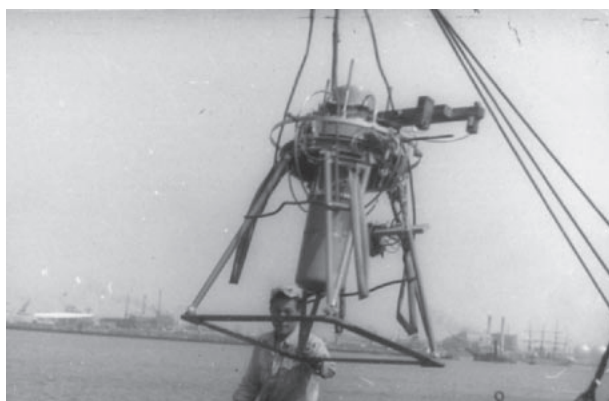
Fig. 5. Loading the bifilar gravity pendulum on "Ryofu-maru". We set up the "bifilar gravity pendulum" in the hold of "Ryofu-maru" of the Meteorological Agency which was anchored in Harumi wharf.
